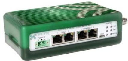
The Xeta-EIO/SIO supports all of the frequencies available from XetaWave now and in the future. Current availability includes the Xeta9 dual band modules for 902 to 960 MHz, Xeta4 narrow band radios for 406-512 MHz, and Xeta24 for the 2.4 GHz ISM band. Future availability will expand to include IO for the Xeta1 (150-232 MHz), Xeta2 (216-232 MHz), and Xeta3 (225-380 MHz).
